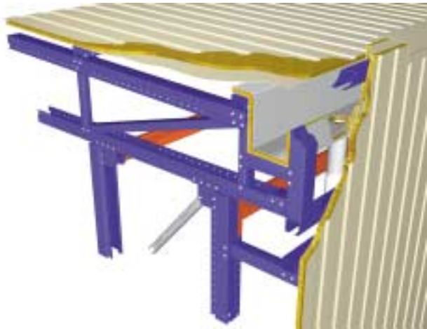
Lower Area of Lateral Cladding
